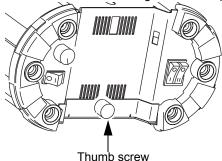
3 Slide the fixture cover open as far as possible (there is a physical stop point that prevents access to the power supply section).
