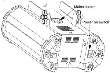
2 Turn the power on using the power-on switch.
